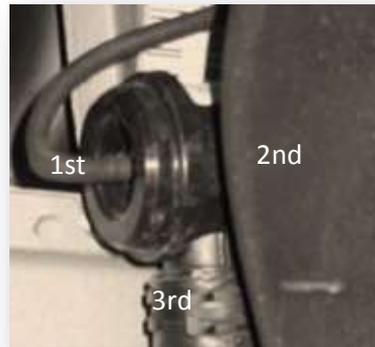
5. You should now have the original dumpvalve removed and can replace it with your uprated dumpvalve. As you can see the Forge Dumpvalve has stronger, more reliable body and internals and piston as opposed to a rubber diaphragm in the original.
